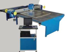
Designed to run 24x7 without sacrificing speed or accuracy, Eastman's Router Tool Head option delivers heavy-duty performance for thick and dense materials. This system offers a two-spindle tool head in addition to the router for a variety of cutting and routing options.
